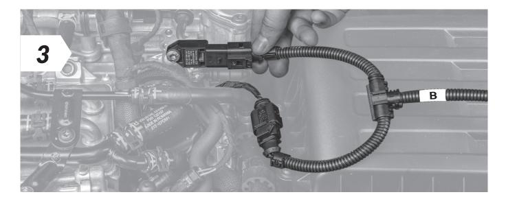
• Now connect the end of the RaceChip wiring harness marked "**B**" to the disconnected connector and the other end to the sensor.
