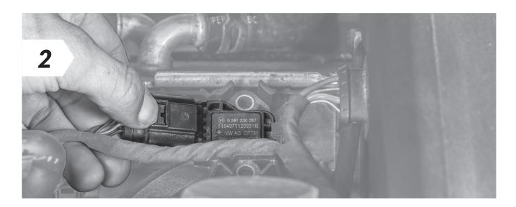
• Disconnect the plug from the manifold absolute pressure sensor.
