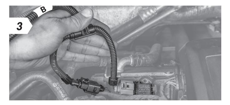
• Now connect the end of the RaceChip wiring harness marked "B" to the disconnected connector and the other end to the sensor.
